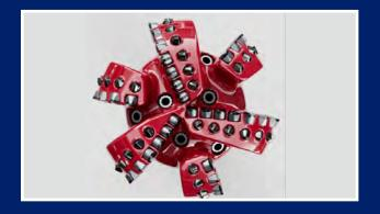
NOV and Particle Drilling Technology are field testing their particle drilling/polycrystalline diamond compact (PDC) hybrid bit designed to provide faster, deeper drilling in hard crystalline rock. An intense stream of hardened particles removes 80-90% of the rock and then the PDC cutters remove the remaining rock and provide stability and a smooth borehole.
