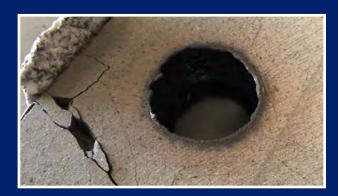
Quaise Energy has designed a millimeter wave drill that is being tested at Oak Ridge National Laboratory. If successful, it will be the first demonstration of drilling a borehole through full rock vaporization. Quaise Energy ultimately aims to reach 10-20 km (6-12 mi) in depth with its drill.
