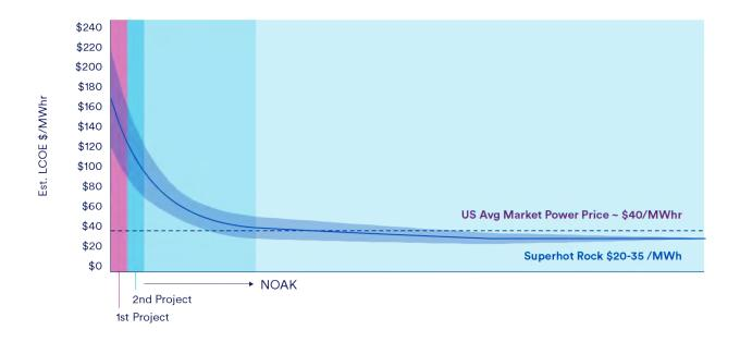
\$20-35 per MWh (Figure 6).<sup>17</sup> Drilling and reservoir development costs—combining labor, equipment, and materials costs—are expected to be higher for first-of-a-kind projects but to progressively decline through continuous improvement, similar to the deep cost reductions and productivity improvements that occurred in large-scale unconventional shale oil and gas development.
