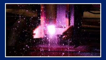
**GA Drilling's** PlasmaBit drilling technology emits a stream of plasma—extreme heat energy formed as electrons are stripped off of atoms using a high-voltage electric current. GA Drilling is currently engineering its drill to operate as a pulsing plasma "hammer." The drill will be powered by a mud-cooled cable, enabling operation in extreme superhot rock temperatures.
