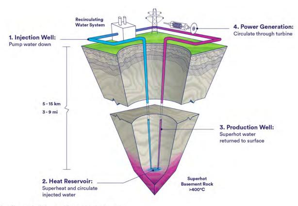
Note: Not to scale. Underground flow conduits for water may either involve below-ground piping or fracture networks (pictured).
