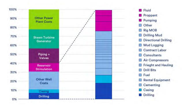
capital cost assumptions. While there are currently significant efforts underway to reduce the cost of drilling, this alone will not push superhot rock energy to a point that it is at grid parity with other producers today. (LucidCatalyst and HERO for CATF, 2022).
